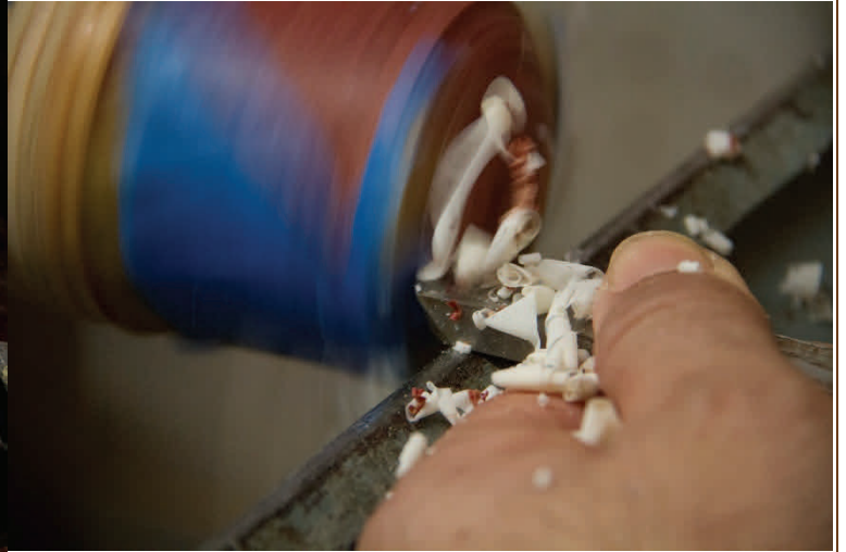
Cured epoxy shaves like plastic when turned, notice the strands of white ribbon peeling away from the manzanita burl wine stopper in progress.
