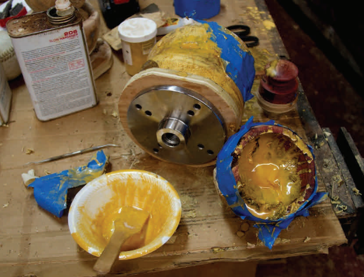
Cured epoxy shaves like plastic when turned, notice the strands of white ribbon peeling away from the manzanita burl wine stopper in progress.
