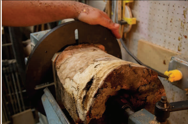
Spalted Copper Beech salvaged from a family estate property. This wood has an amazing array of coloration and detail caused by deterioration.
